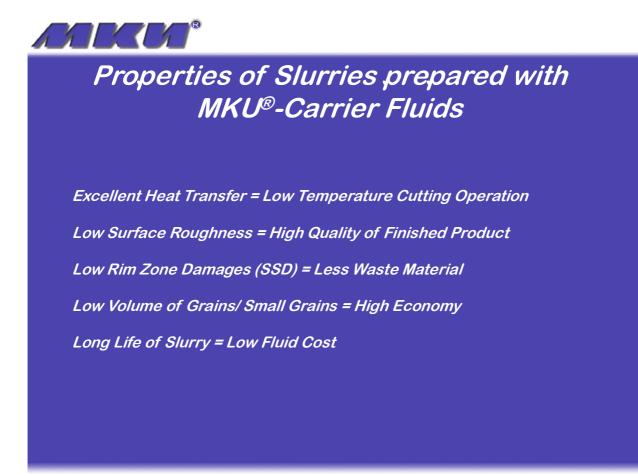
Connected to the last point it is particularly important that slurries prepared with MKU<sup>®</sup> Fluids show no tendency to form hard sediment conglomerates, even not after long resting periods.
