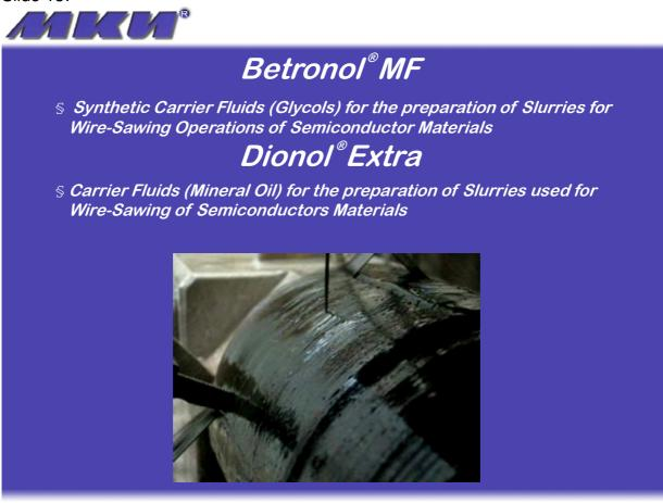
The individual carrier fluids are distinguished by their formulations corresponding to the different process parameters as e.g. grain size, grit proportion, speed of wire, diameter of wire and diameter of ingot.
